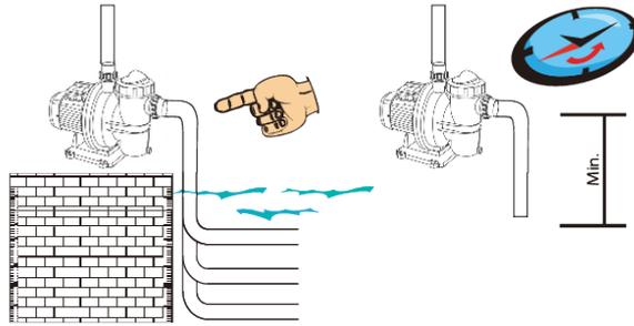
GB If there are several suction pipes, arrange the pipes and the manifold below water level and reach the pump with only one vertical pipe.
