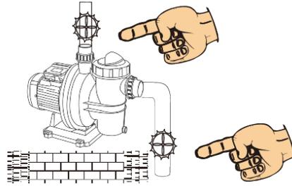
GB Fit one gate valve in the suction pipe and one in the delivery pipe to isolate the pump.
